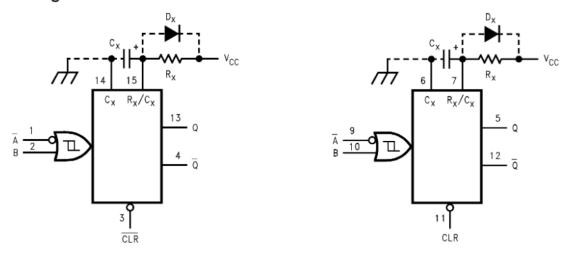
Note A: C<sub>x</sub>, R<sub>x</sub>, D<sub>x</sub> are external Capacitor, Resistor, and Diode, respectively.
