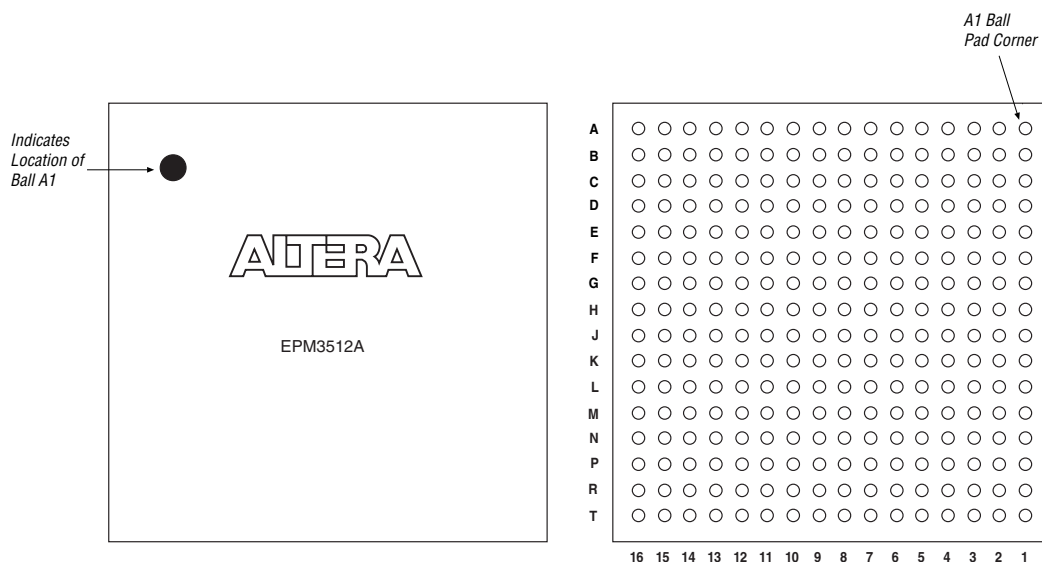
Figure 18. 256-Pin FineLine BGA Package Pin-Out Diagram
